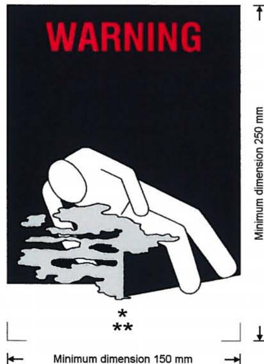
Coolant/conditioning warning mark for wagons and containers
