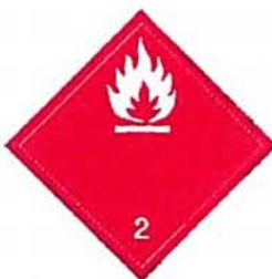
(No. 2.1) Flammable gases Symbol (flame): black or white (except as provided for in 5.2.2.2.1.6 (d)); Background: red; Figure "2" in bottom corner
