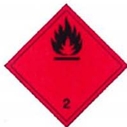
(No. 2.1) Flammable gases Symbol (flame): black or white (except as provided for in 5.2.2.2.1.6 (d)); Background: red; Figure "2" in bottom corner
