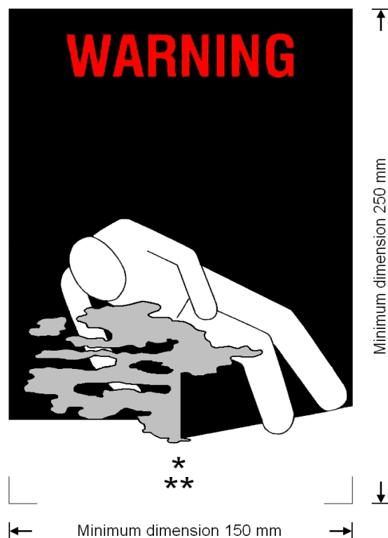
Coolant/conditioning warning mark for wagons and containers
