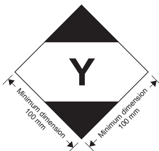
Mark for packages containing limited quantities conforming to Part 3, Chapter 4 of the ICAO Technical Instructions
